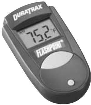
The DuraTrax® FlashPoint™ Temperature Gauge is a non-contact infrared thermometer. Specifically designed for use with R/C engines, batteries, motors, sealing irons and heat guns, simply aim the temperature gauge at the target and press the measurement button to quickly and easily display the surface temperature! The distance to target ratio is 1:1, and therefore the temperature gauge should be positioned as close to the target as possible.
