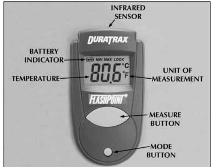
Sometimes it is easier to accurately measure the temperature of an object by physically attaching a thermometer or thermocouple to it. However, it can often be difficult or inconvenient to do so. Sometimes, it is only necessary to see the large heat patterns of an object, rather than measuring a temperature at a very precise location on the device. In these cases, measuring an object's heat radiation with an infrared temperature gauge is a good solution.
