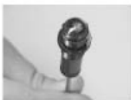
STEP6, Fill oil to the top and keep the shock body vertical. Do not use oil weight too high.
