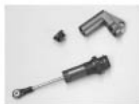
STEP4, Remove the piggyback and the piggyback bottom cap
