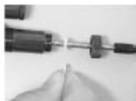
STEP2, It's possible to replace thick stock washer with a thinner one for smoother o-ring actions
